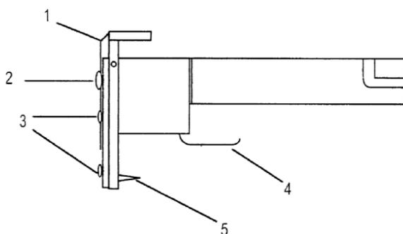
Figure 8: De-capper head assembly
